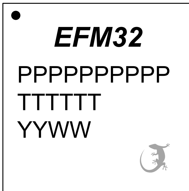
Figure 6.3. BGA120 Package Marking
