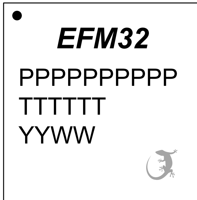
Figure 8.3. TQFP100 Package Marking
