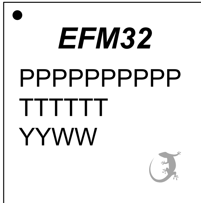
Figure 10.3. QFN64 Package Marking
