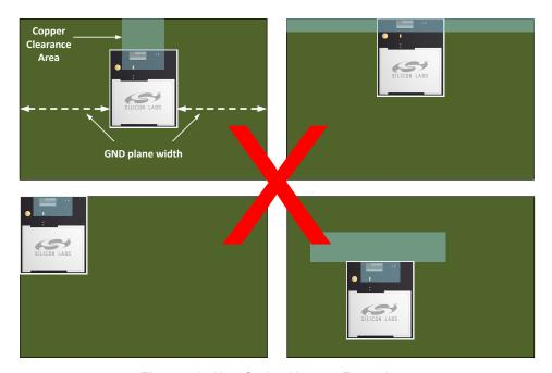
Figure 7.3. Non-Optimal Layout Examples
