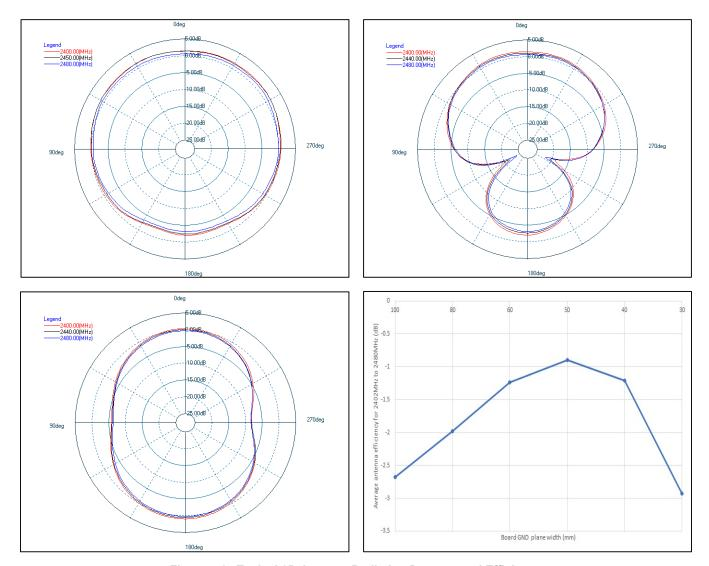
Figure 4.1. Typical 2D Antenna Radiation Patterns and Efficiency
