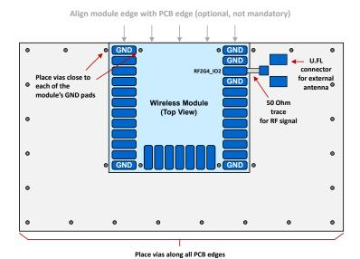
Figure 7.2. Recommended Layout for MGM210P Using External Antenna
