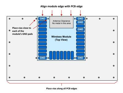
Figure 7.1. Recommended Layout for MGM210P Using On-Board Chip Antenna
