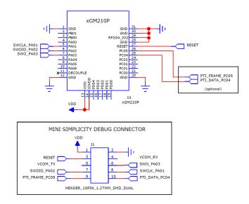
Figure 5.2. Stand-Alone SoC Configuration
