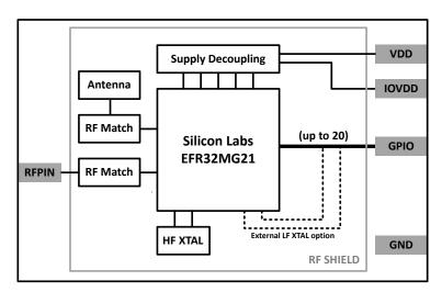
Figure 3.1. MGM210P Block Diagram
