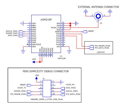
Figure 5.3. Stand-Alone SoC Configuration with External Antenna
