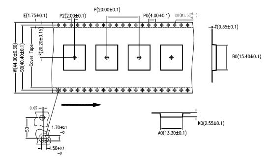
Figure 10.1. Carrier Tape Dimensions
