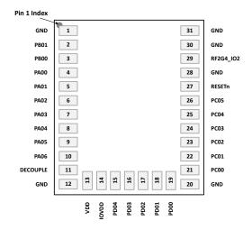
Figure 6.1. MGM210P Module Pinout
