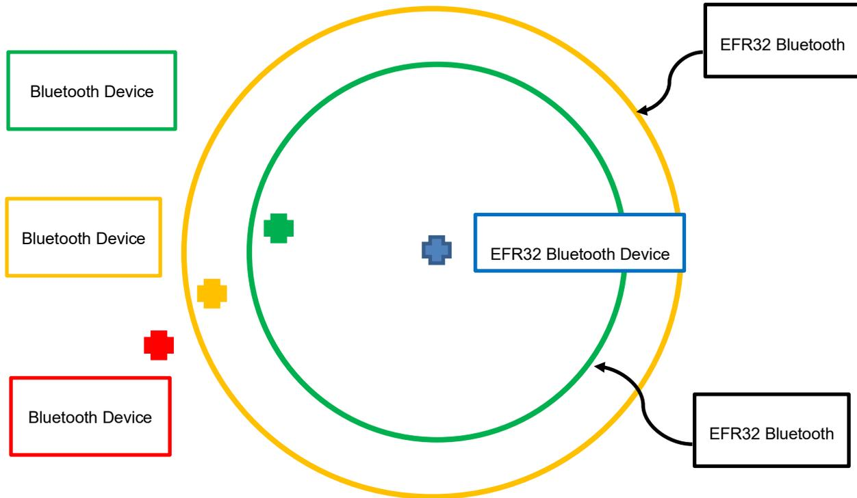
Figure 2-3. EFR32 Receiver Desensitized when Wi-Fi Transmitting
