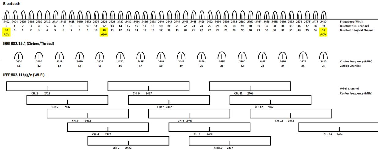
**Figure 2-1. Wi-Fi, Bluetooth, and 802.15.4 Channel Mapping (World-Wide)**
