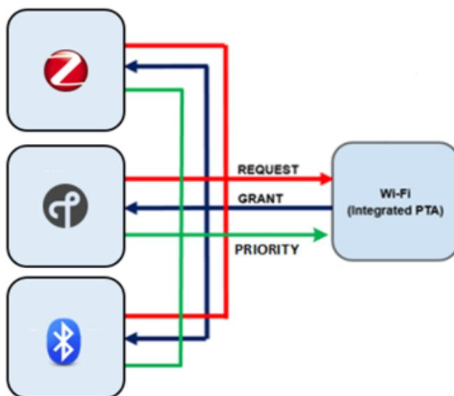
**Figure 4-4. Three EFR32s Supporting Single Wi-Fi/PTA 3-Wire PTA Interface**
