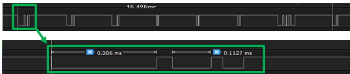
Figure 4-5. High-Duty Cycle Wi-Fi TX Active
