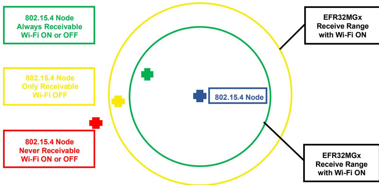
Figure 2-5. EFR32MGx Receiver Desensitized when Wi-Fi Transmitting
