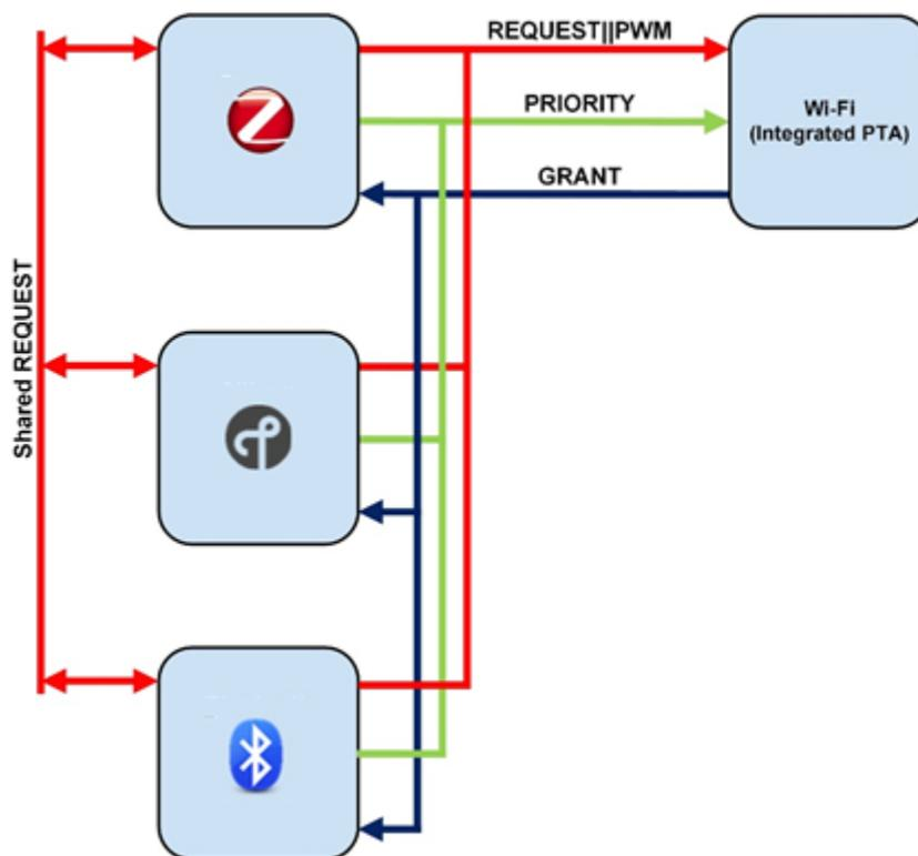
**Figure 4-7. Three EFR32s Supporting PWM and Wi-Fi/PTA with Single 3-Wire PTA Interface**
