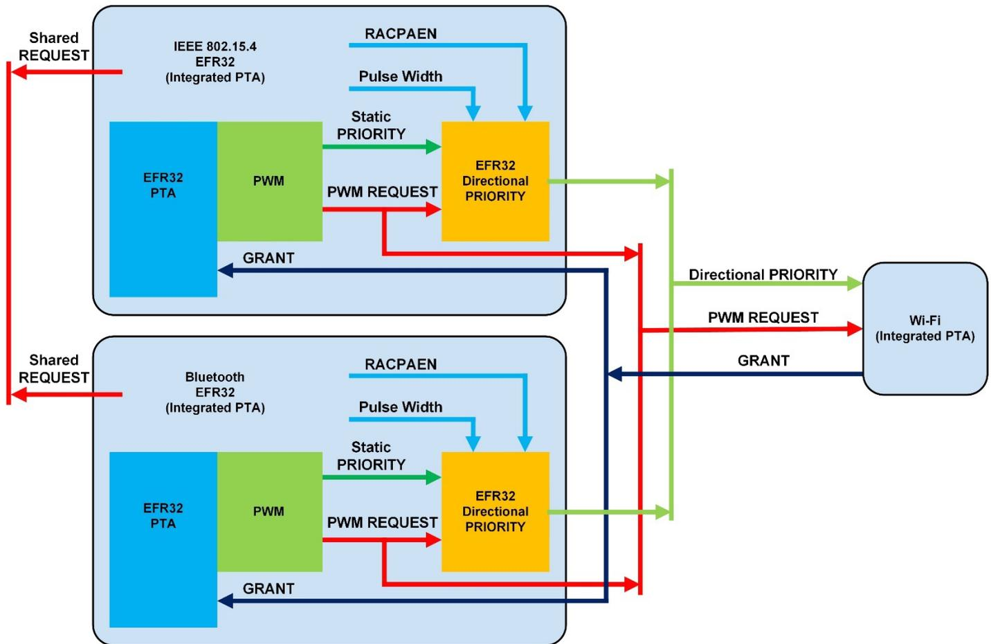
Figure 4-10. Multi-EFR32 PTA with SDK PWM and Directional PRIORITY
