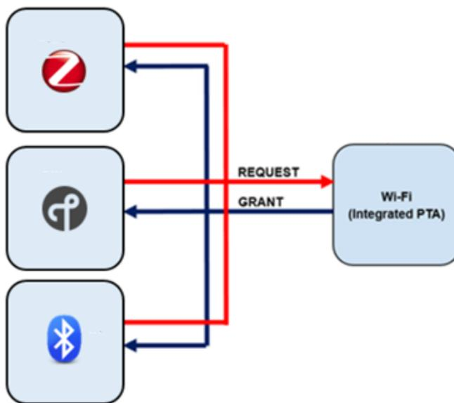
**Figure 4-3. Three EFR32s Supporting Single Wi-Fi 2-Wire PTA Interface**
