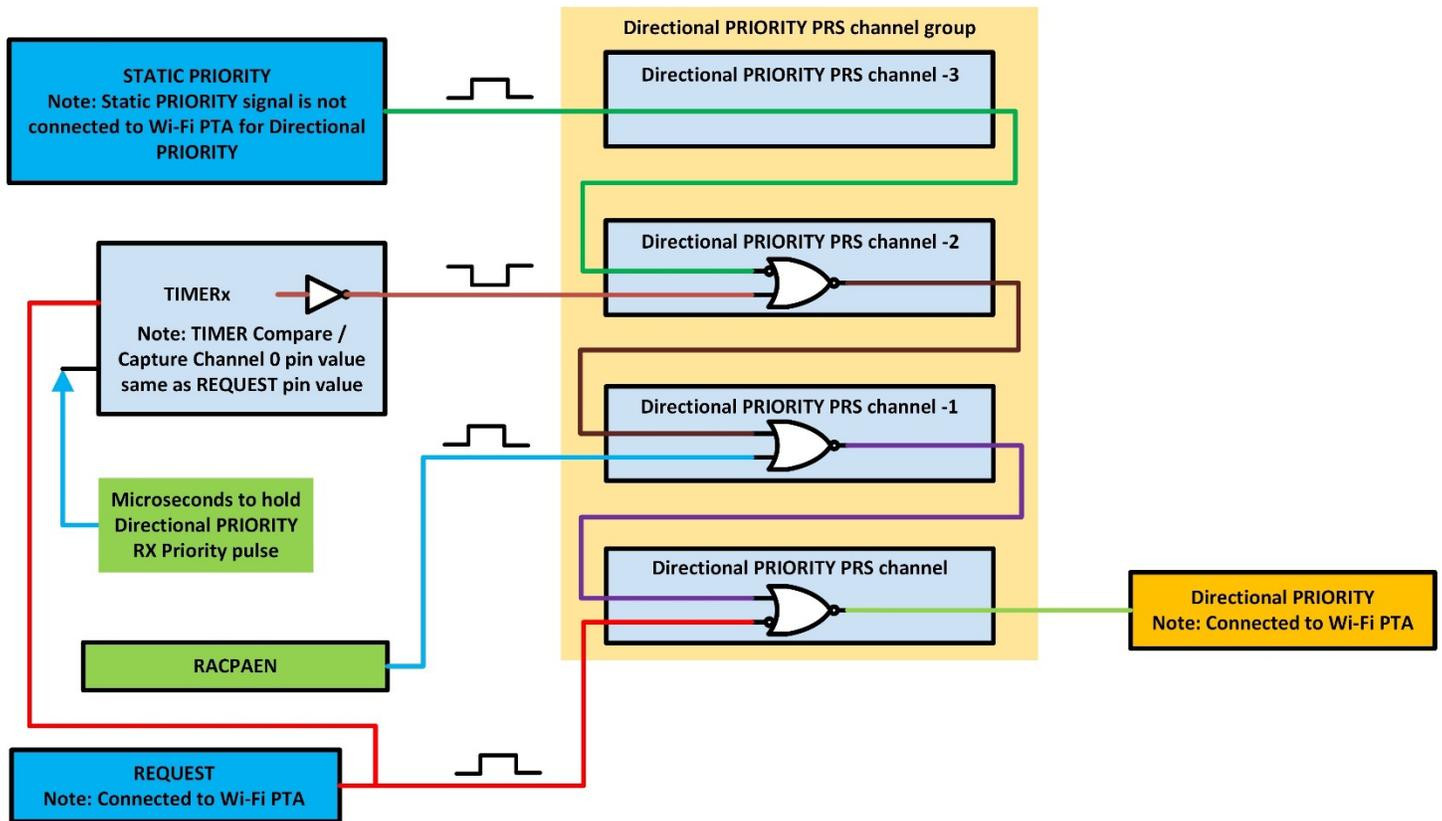
Figure 4 12. EFR32xG2x Directional PRIORITY Logic Diagram
